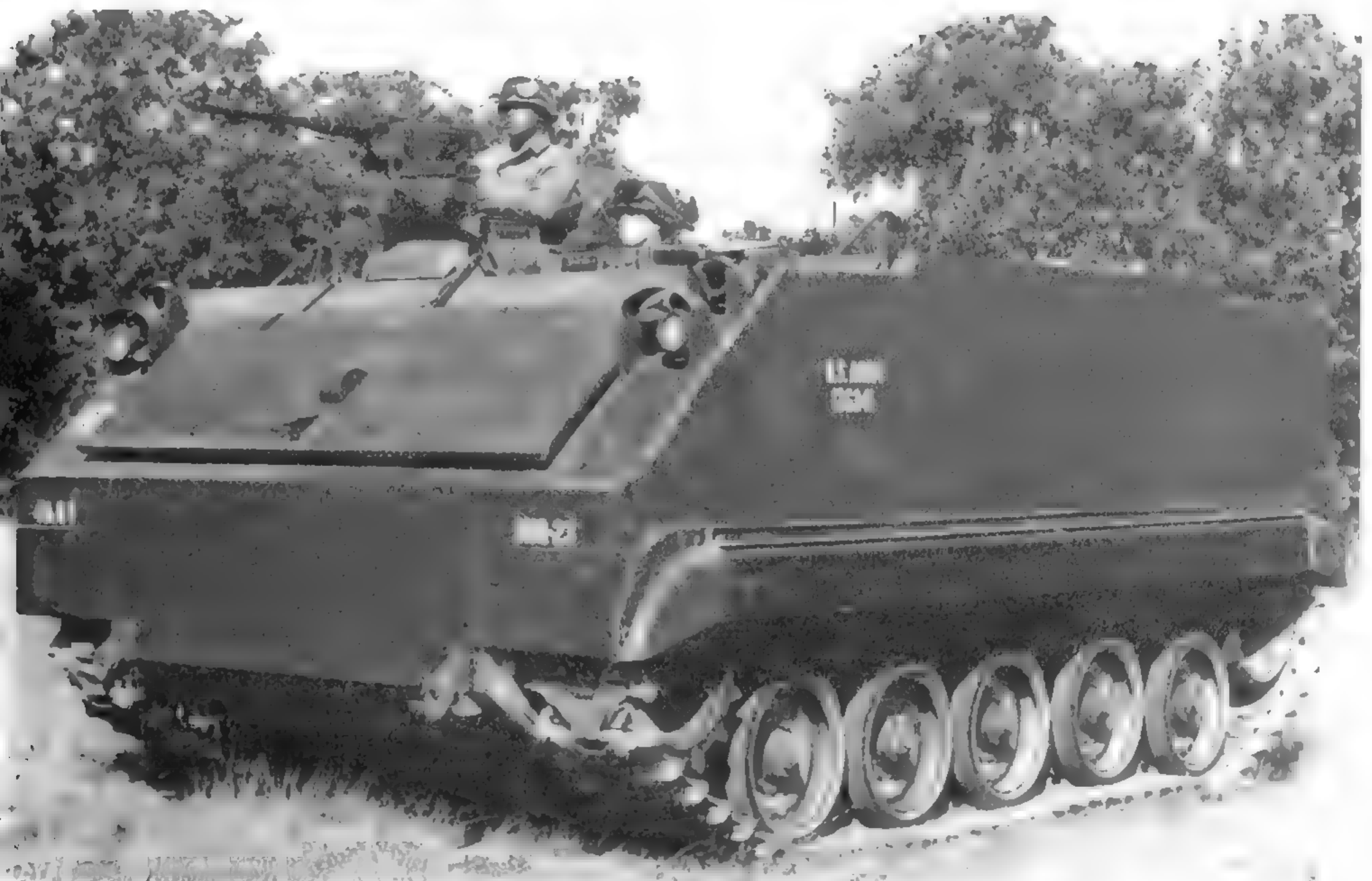
Shown in this October 1961 photograph is an early production M59 armored personnel carrier. Notice the commander's machine gun is mounted externally to the cupola. The trim vane, necessary for amphibious operations, is shown stowed against the front of the hull. (U.S. Army photo)
